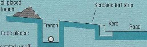
Try to limit the time trenches are open to fewer than three days and avoid opening them whenever the risk of storms is high. Remove and store vegetated topsoil (sod) so that it can be used to provide immediate erosion protection after backfilling.
