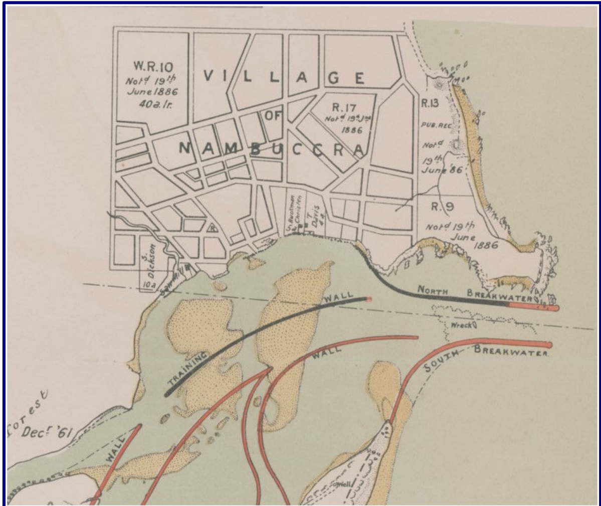
Figure 2 – Construction of the Nambucca River Breakwaters Extract from The Department of Public Works Plan of constructed (black) and proposed works (red) for the Nambucca River breakwaters and training walls – 30 June 1902.
