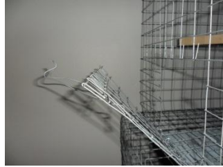
Tie wire hooks for the door.
