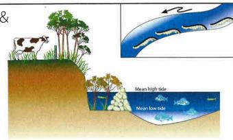
Applicable where a suitable bench exists in front of the eroding bank, this technique is designed to reduce the effect of waves on susceptible riverbanks, and allows mangrove and reed establishment on the intertidal foreshore. Rock embayments are constructed to just above mean high water mark. They are keyed into the bank at the upstream end then run parallel to bank and are open downstream. Similar cost to rock revetment.
