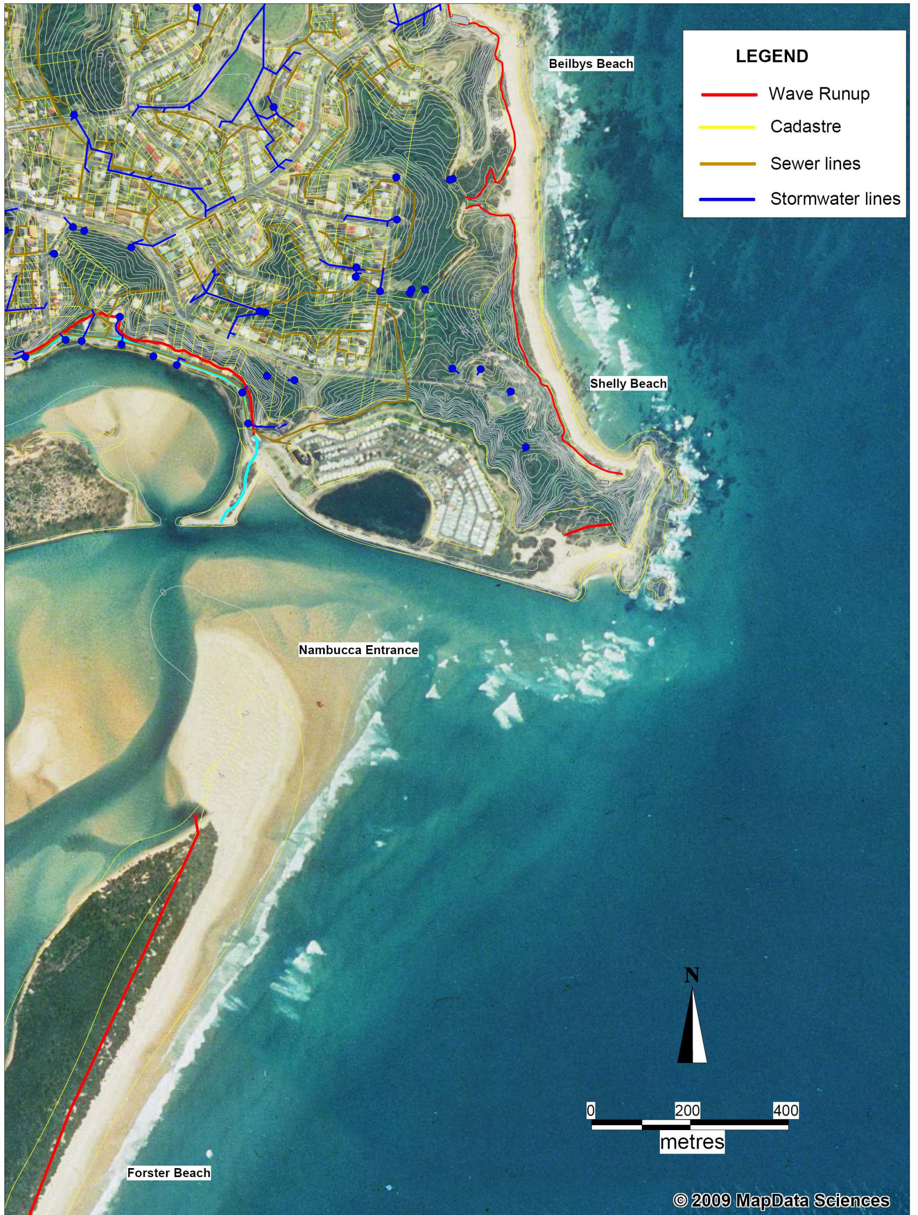
Figure 4.7a – Wave Runup limits, Nambucca entrance, Shelly Beach and Beilbys Beach, Nambucca Heads
