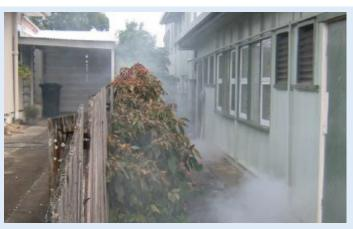
Smoke testing used to pinpoint the places where stormwater is entering the sewerage network.
