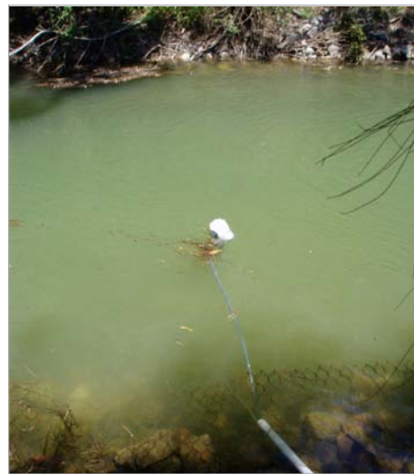
Plate 2 Suction line for sampling estuarine
