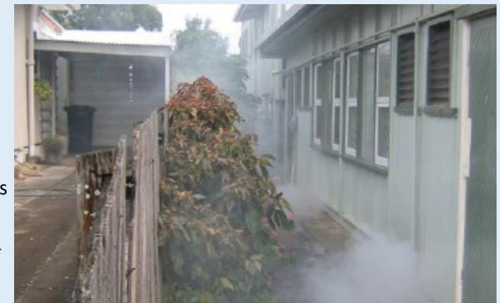
*Smoke testing used to pinpoint the places where stormwater is entering the sewerage network.*
